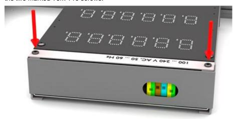
The protective ground wire (yellow/green) can be connected either to the yellow or the green terminal.
