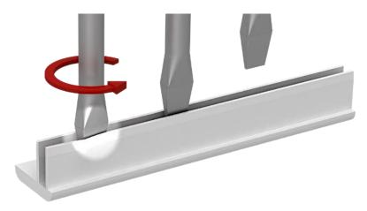
Insert the front pane and the connectors. Spread the connectors slightly with a screwdriver before inserting so that they are stuck firmly in the housing frame. Check that the connectors are fixed so tightly after insertion that they cannot be removed without tools (lever tools).
